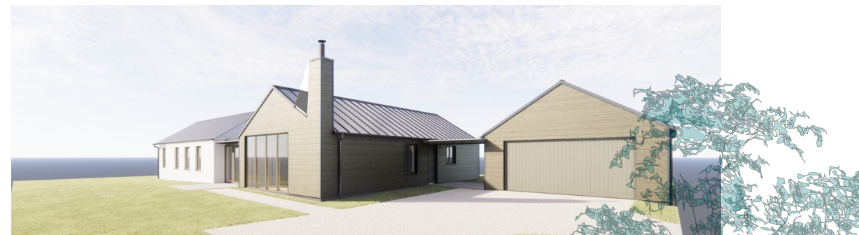
ABOVE - proposed image of cottage front approach showing double gables pitched roof with height and angle to match existing cottage and chimney to corner
